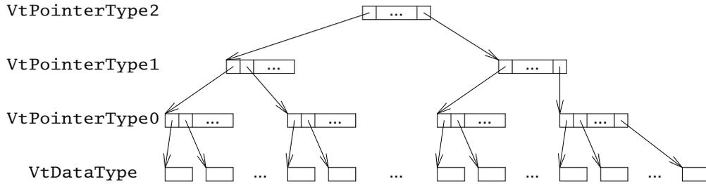
The leaves are the original data stream. Those blocks have type `VtDataType`. The first pointer stream has type `VtPointerType0`, the next has type `VtPointerType1`, and so on. The figure ends with a single block of type `VtPointerType2`, but in general trees can have height up to `VtPointerType6`. For a *dsize* of 8192 bytes and *psize* of 8180 bytes (409 pointers), this gives a maximum stream size of approximately 10 zettabytes ( $2^{73}$  or  $10^{22}$  bytes).
